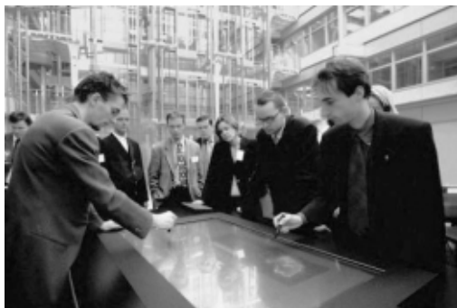
The InterTable supports stand-up meetings of small groups. The 50" monitor provides digital information via a touchable surface. (Design: Wilkhahn, Fraunhofer-IPSI, Andreas Störiko.)
