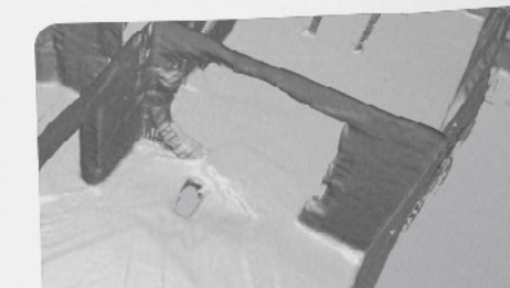
Photogrammetry detects different openings in the walls (doors/windows) and in the floors (holes)
